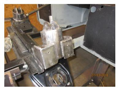
I wanted to make the top wishbone longer but space was limited. I angled the top wishbone a few degrees down towards the centre line, which proved to be a mistake. I thought that placing the coilover mount in the lower wishbone in
