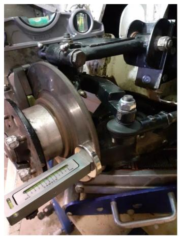
The next issue was to remount the steering rack to remove the severe bump steer. The rack had to be lowered and mounted onto the top of the chassis legs, which necessitated new steering arms to be made, from EN16 steel, about 3/8" sawn off the ends of the track road and the threads ends extended. As you can see, install had to two universal joints in the I made up a column. brace bar to bolt on either side of the turrets - the
