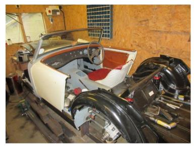
The front H section chassis legs and one piece floor pan were bolted to the risers. Gradually the shell constructed. the was horizontal jig rails giving a datum permanent measure from. together with the vertical datum, using a spirit level. I used fibre glass front wings, bonnet and one piece tail, the shell would be as light
