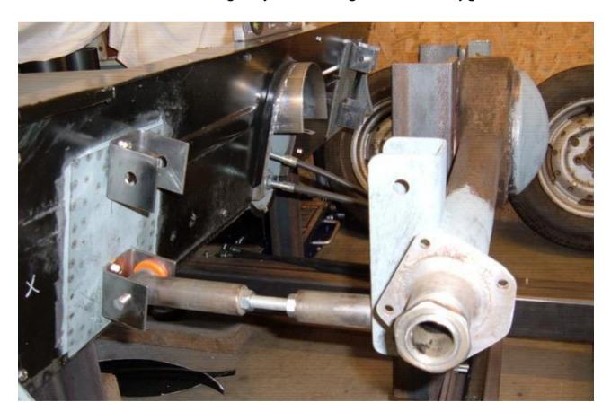
Radius arm mountings with adjustable arm to determine final lengths, with axle tube bolted to jig,
