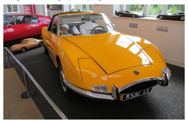
Matra M530 powered by a Ford V4 1700 cc engine which was mid mounted with a transaxle
