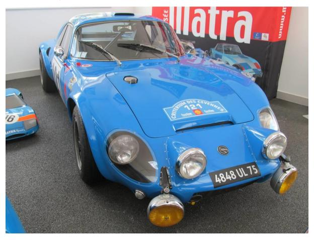
1965 Matra M610 rally car Cosworth Ford Twin Cam engine, Hewland gearbox, 645kg 145 bhp
