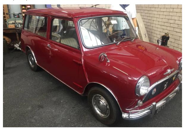
Left hand drive prototype Mini Traveller with an 848cc engine used for testing in Switzerland
